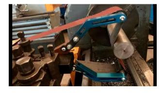
An interesting tool for sanding and finishing parts easily and safely on conventional lathes. Conceived in accordance with ISO23125 Standards 6.2.1 (no use of hands during working operations).
